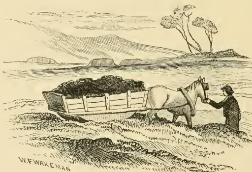
FIG. 37.—Slide car, still occasionally used for drawing weights over soft ground.
